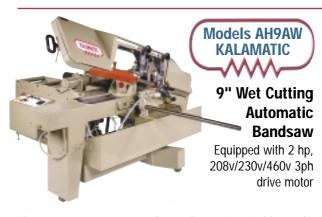
Operators can set-up the Kalamatic quickly and the procedure is easily learned. The feed roller and saw head is lifted, stock loaded and positioned, stock stop adjusted for proper length, the number of pieces required is entered in the counter and then the cutting cycle is initiated by the operator. After that, the saw operates automatically until all pieces are cut or the stock is exhausted.
